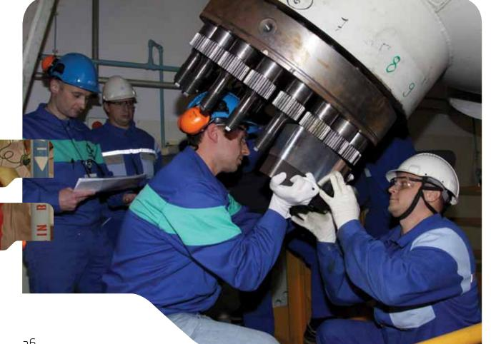
Predictive maintenance included establishing equipment status on the basis of various techniques not part of the primary maintenance thermographic inspection, vibration inspection of major rotating components, lubricant quality inspection, and the inspection of rotors during the operation of high-power electric motors.
